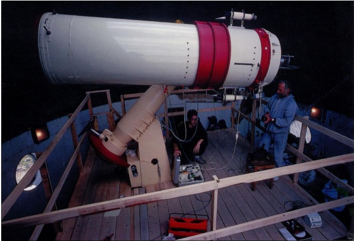
Figure 18: The 62-cm telescope that replaced the coronagraph in the 7-m dome at Saint Véran (courtesy: Paris Observatory).
